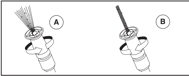
Figure 15: Adjusting the nozzle for spray pattern
